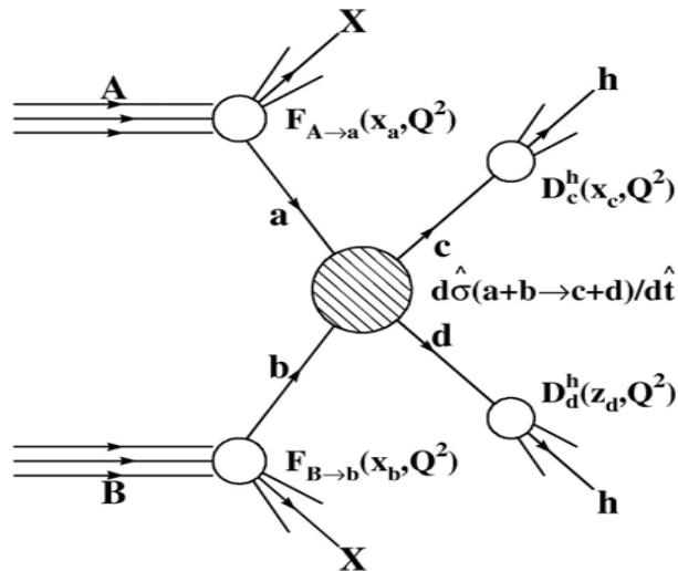
$$\sigma = \sum_{a,b} \int dx_a dx_b f_a(x_a, Q^2) f_b(x_b, Q^2) \hat{\sigma}_{ab}(x_a, x_b)$$
